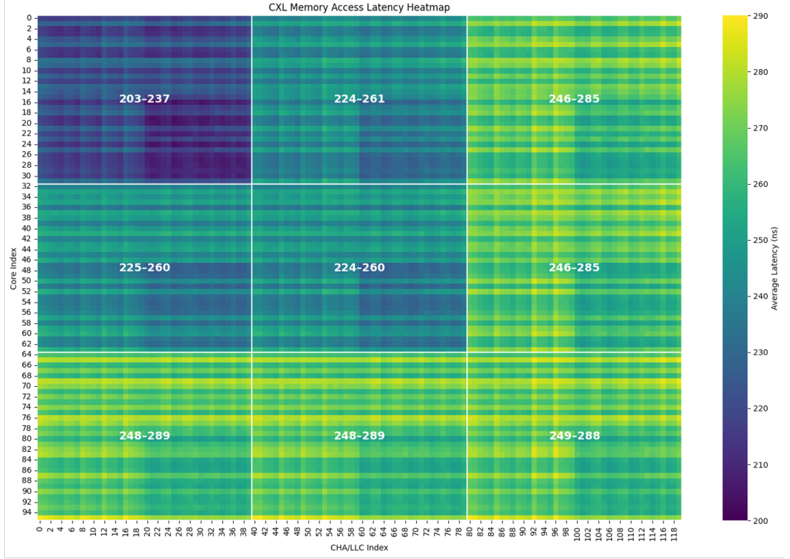
Figure 3.7: CXL latency broken down by path taken by requests within processor. The CXL device is attached to the IO die that is physically closest to the compute die containing cores 0 – 31 and CHA slices 0 – 39.
